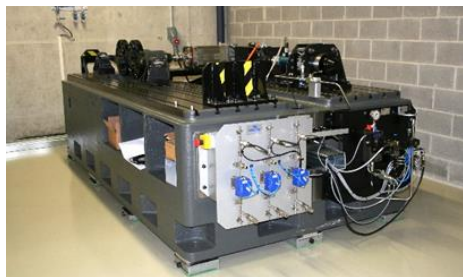
Pilot for tribological testing of seals
