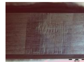
Seal degradation in laboratory tests
